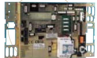
OPTIONAL CB 12 INTERFACE CARD It features more connectors than the CB card for greater modularity. (Voltage protection option mounted (CM606))
